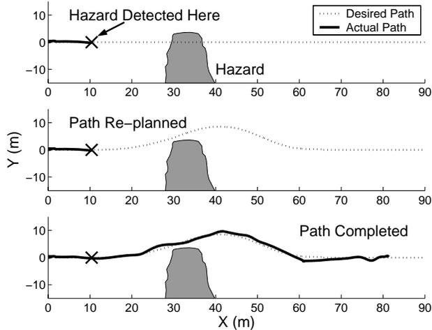
Figure 18. Rough terrain experimental results.
