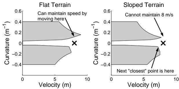
Figure 14. Trajectory space comparison for flat and sloped terrain.
