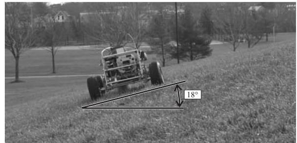
Figure 13. Image of ARTEmiS sloped terrain experiment.
