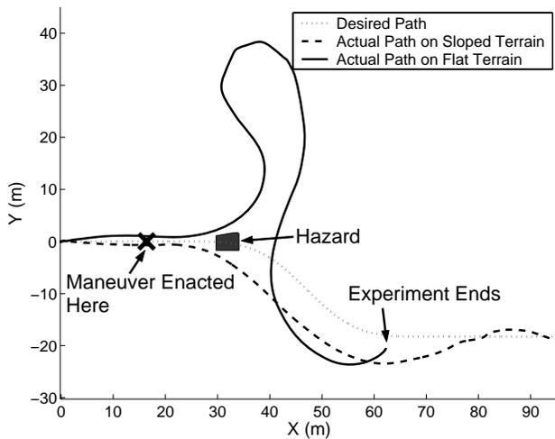
Figure 15. Hazard avoidance maneuver enacted on flat and sloped terrain.
