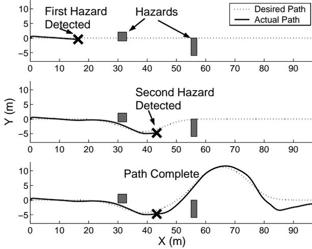
Figure 11. Hazard avoidance maneuvers executed for multiple hazards.
