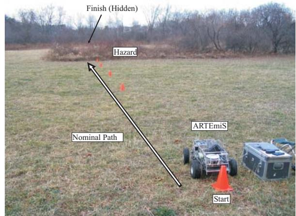
Figure 17. Rough terrain experimental setup.
