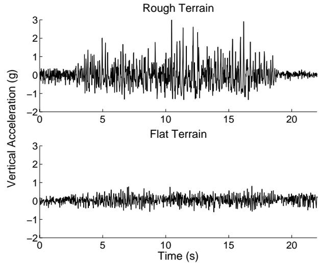
Figure 16. Vertical acceleration comparison on rough and flat terrain.
