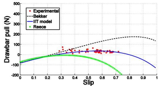
Fig. 6: Drawbar pull versus slip with the shifting mass at the centre of the VIV
