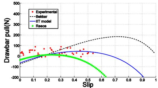
Fig. 7: Drawbar pull versus slip with the shifting mass at the rear of the VIV
