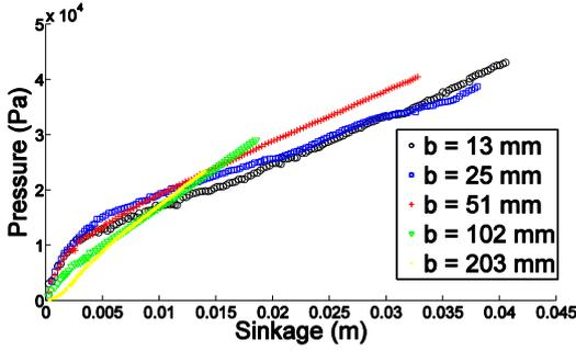
Fig. 13: Width dependence for a 178 mm diameter wheel on dry quartz sand
