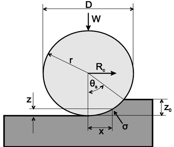
Fig. 1: Wheel pressure sinkage geometry
