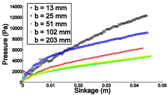
Fig. 11: Width dependence for a 267 mm diameter wheel on a clay/silt mix
