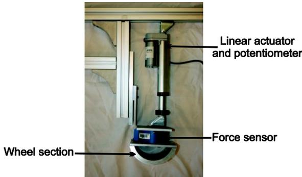
Fig. 8: Pressure-sinkage testbed
