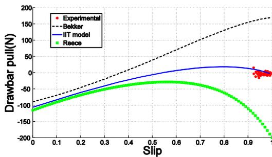
Fig. 5: Drawbar pull versus slip with the shifting mass at the front of the VIV
