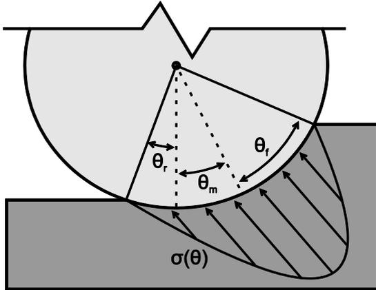
Fig. 2: Normal stress distribution beneath a wheel
