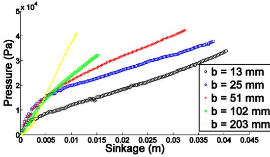
Fig. 14: Width dependence for a 267 mm diameter wheel on dry quartz sand
