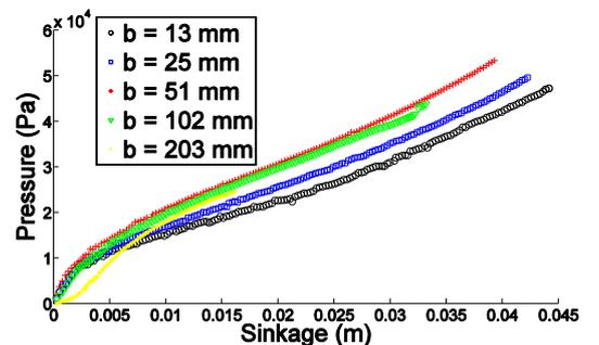
Fig. 12: Width dependence for a 114 mm diameter wheel on dry quartz sand
