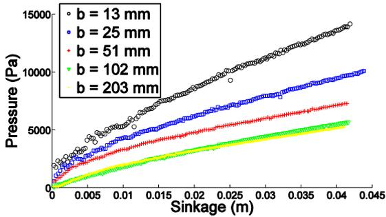
Fig. 10: Width dependence for a 178 mm diameter wheel on a clay/silt mix
